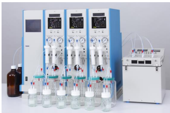
FMS EconoTrace SPE with SuperVap concentrator, the system can run up to 8 samples simultaneously
