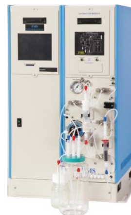
Figure 3. TurboTrace for SPE of diethylene glycol/water samples.
