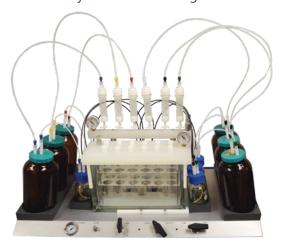
Using vacuum & nitrogen, the EZSpe automatically loads the samples, rinses the sample bottle and delivers the solvent to the SPE cartridges. The analytes of interest are extracted and then dried using a sodium sulfate cartridge to remove all water. The final extract can be delivered directly to the "Direct to GC vial Vessel" ready for final concentration in the FMS SuperVap®. The process saves both labor and time.
